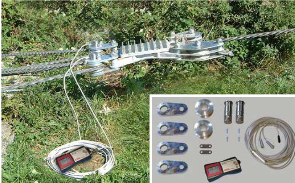
Electronic tension measurement device with measuring pins.
