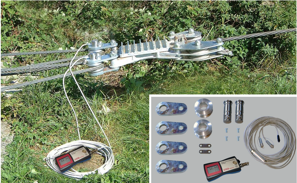
Electronic tension measurement device with measuring pins.
